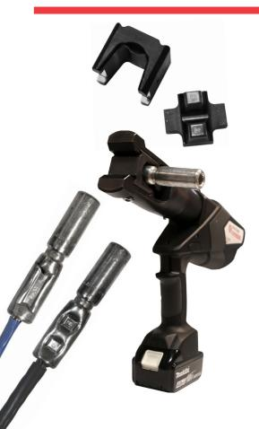
Unique system for aluminium crimping in the 1300 system. The system is designed for low voltage applications (1 kV) and is adapted for groundcovered cable. The number of punches and matrixes has decreased from the previous 21x (including prerounding) to 3 punches and 3 matrixes for the indent crimping of both round and sector-shaped Al conductors in the range 50-240 mm<sup>2</sup>.
