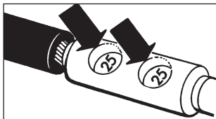
Example of an identification mark that the punch leaves behind on a cable connector.
