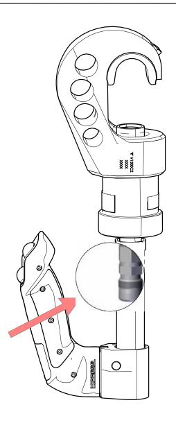
Risk for oil leakage in the quick coupling, see the area the arrow shows. It's is very important that the Ergo pipe is not loosen and it has it's original position to prevent sudden oil leakage.
